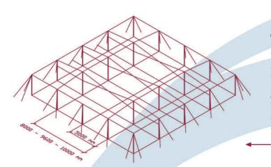
This Net House is a structure consisting of galvanised hollow sections, steel wire and strand and covered with mesh metal. It can be adapted to any kind of ground and shape to get a high profit rate. It is suitable for dry regions snd can include zenithal ventilation. Suitable for DRY regions.
